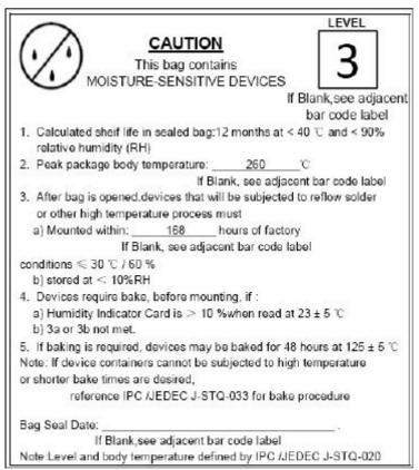
The module Must go through 125℃ baking for at least 9 hours before SMT AND IR reflow process!
